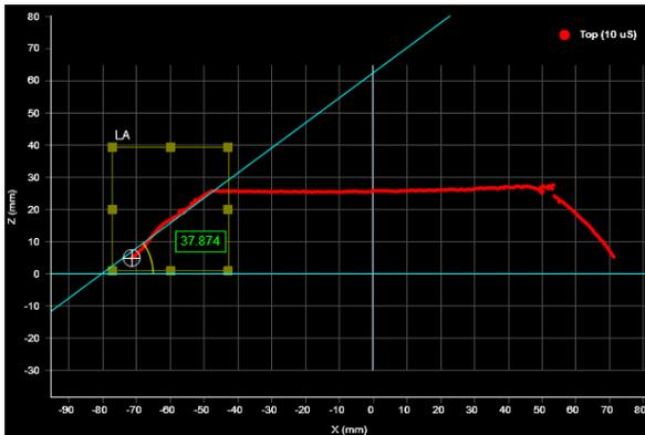
Curve of upward-facing wane detected as larger angle: PASS.
